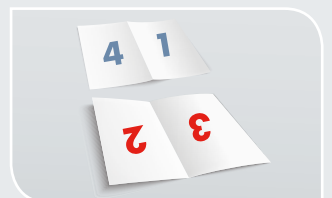
Check for correct print direction
