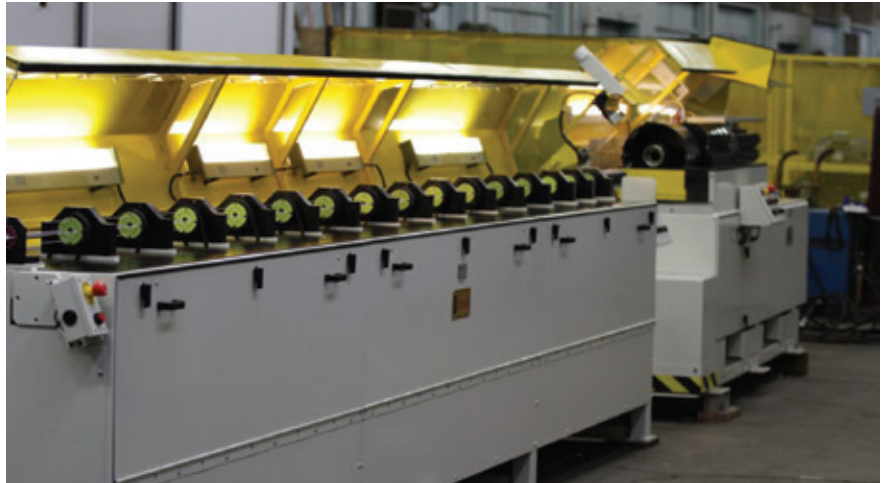
▲ A rebuilt Tensor SZ strander with state-of-the-art electronics
