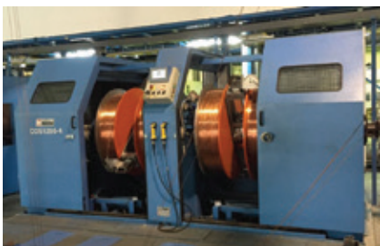
▲ A power regenerative high speed concentric strander module of four reels with three wires each (Pourtier COS 1200-4)
