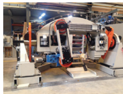
▲ A large double twist stranding/laying-up machine (Setic TC 1250-4M)
