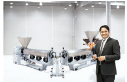
▲ The solar cable co-extrusion line from RosendahlNextrom
