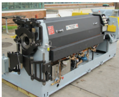
▲ A rebuilt 150mm (6") Davis-Standard rubber extruder
