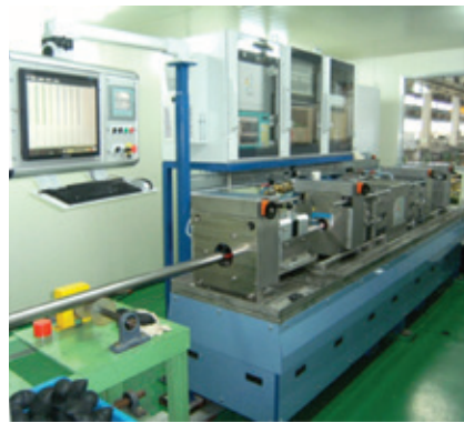
▲ Complete titanium tubes inspection by UT and ET
