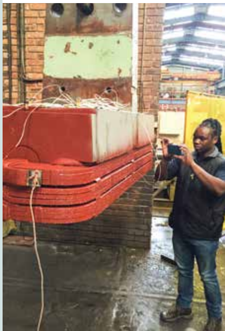
Marthinusen & Coutts' rotating machines design engineer, David Motloung, records photographic evidence of tests on one of the enormous gearless mill drive rotor poles recently refurbished by the company.
