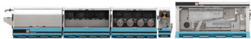
○ Electronically controlled MSM 85 type rod breakdown machine with integrated RA 501 continuous annealer
