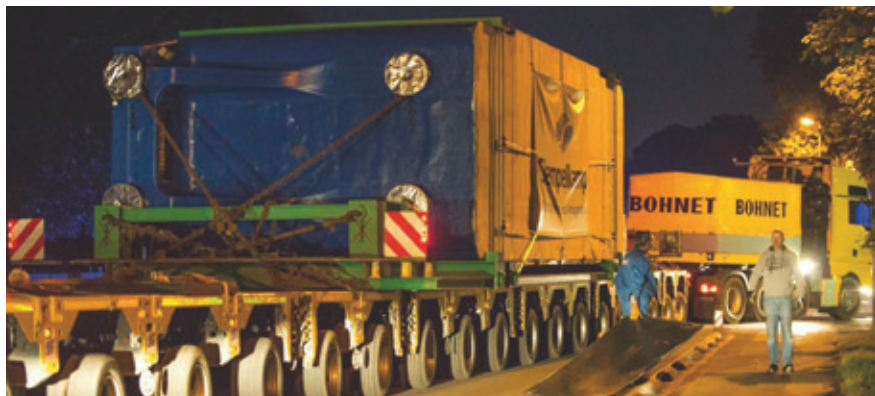
○ The towing and push-back vehicles together weigh 70 tonnes. On top of that, the trailer (50t) and the press component part (maximum 287t) add up to a total weight of more than 400 tonnes
