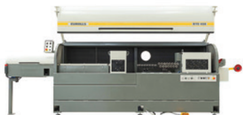
○ New RT600 straightening and cutting line for electrodes
