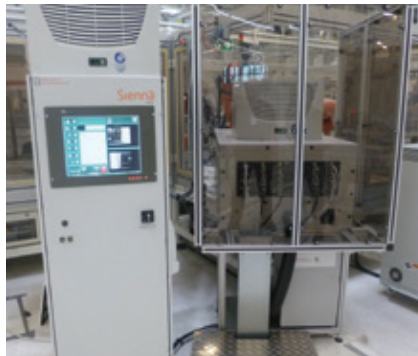
○ Spectrum Technologies' Sienna 900 laser magnetic wire pulling system was chosen by Volkswagen AG
